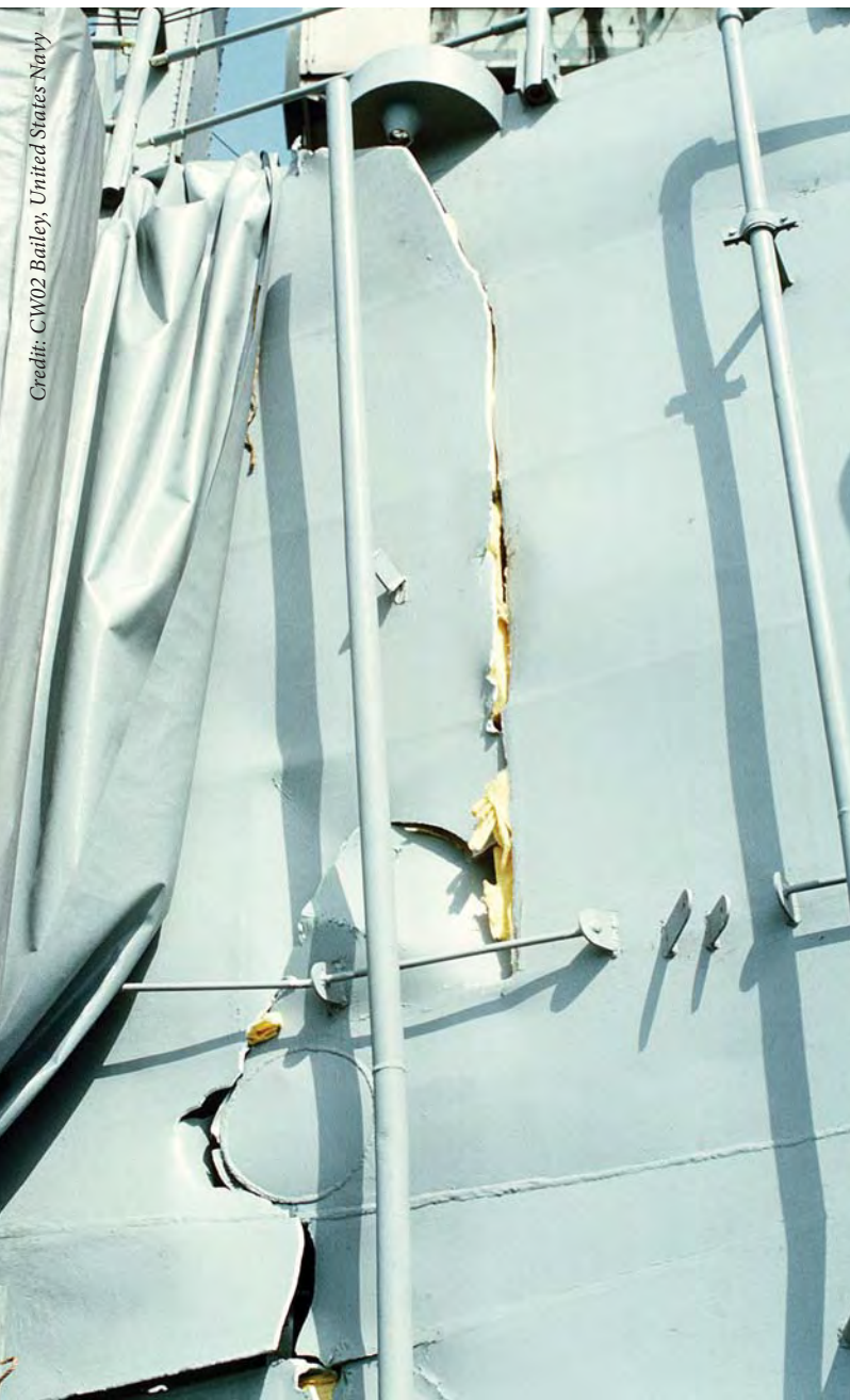
A crack runs through the superstructure of the Aegis cruiser USS Princeton following a mine strike during Operation Desert Storm . Photographed 21 February, 1991. HMCS Athabaskan was requested to escort Princeton out of the mine field.
