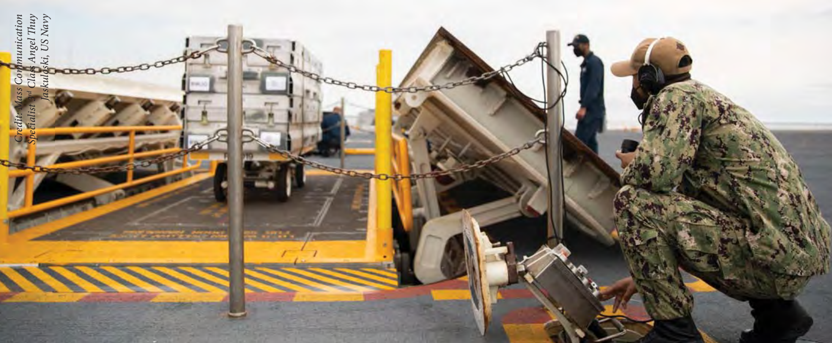
A sailor on USS Gerald R. Ford operates one of the ship's advanced weapons elevators during a post-delivery test and trial period in April 2021. Ford's elevators have required extensive troubleshooting as they utilize new technology and are emblematic of the first-of-class issues with the Ford -class.
