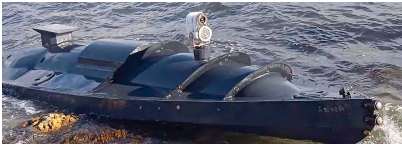
A Ukrainian 'kamikaze drone' is spotted beached on the Crimean coast, October 2022. The propulsion system purportedly matches the one produced for Bombardier's Ski-Doo recreational vehicles.
