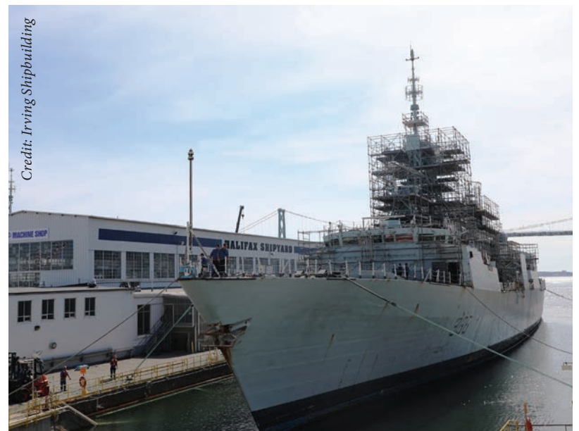
HMCS Montreal enters Halifax Graving Dock to begin a 53-week Docking Work Period. Maintenance and refit is an oft-overlooked component of the National Shipbuilding Strategy.
