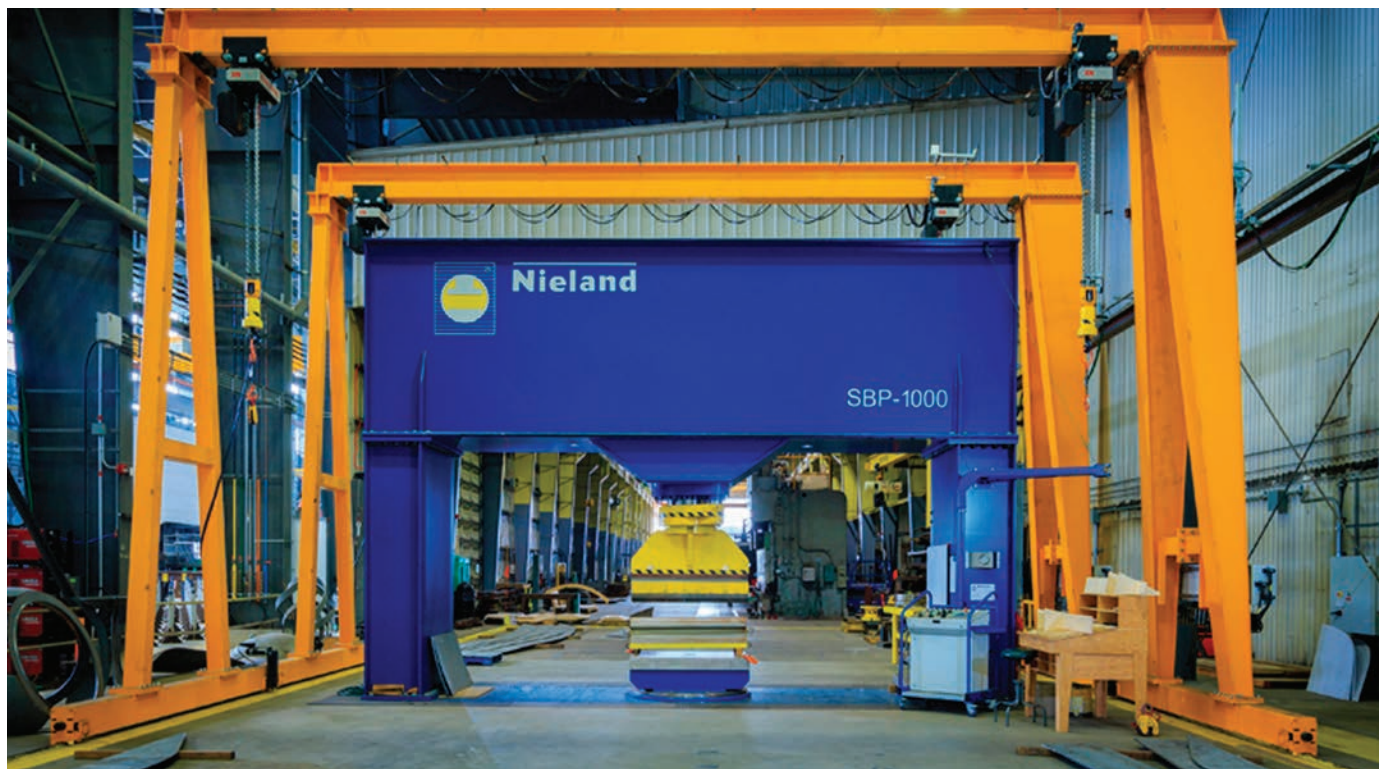
The 130 metre long Forming Shop is one of the legacy buildings at Seaspan Vancouver Shipyards predating the NSS modernization. Nonetheless, it is home to some of the yard's most advanced equipment, such as this 1000t hydraulic plate press that can bend 2.5"-thick steel plates.
