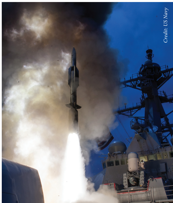
USS John Paul Jones fires an SM-6 missile on 19 June 2014, during a series of live-fire tests. The SM-6 is the latest variant of the Standard Missile family, designed to receive guidance data from external sensors to enable the missile to engage targets well beyond the launch vessel's own sensor range.
