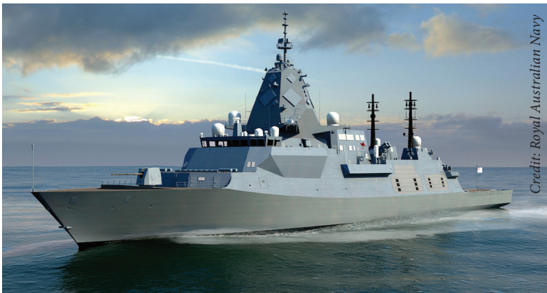
The Australian version of the Type 26, the Hunter -class, features the domestically-produced CEAFAR 2 phased-array radars combined with the American Aegis Combat Management System.
