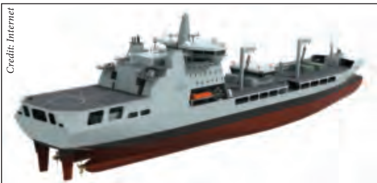
The Tide -class tankers are a proposed class of four large fast fleet tankers for the Royal Fleet Auxiliary (RFA) of the United Kingdom. Here is an artist's conception of the BMT Defence Services' AEGIR tanker concept.
