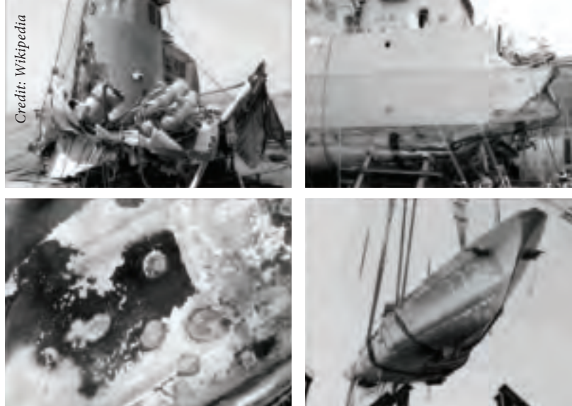
Damage to ROKS Cheonan after being hit by a North Korean torpedo in March 2010 — clockwise from upper left: (1) "stack-damage"; (2) front portion (port side) of ship showing the break point; (3) front half of Cheonan as a large fragment is lifted from the sea; (4) water pressure marks on the hull bottom.
