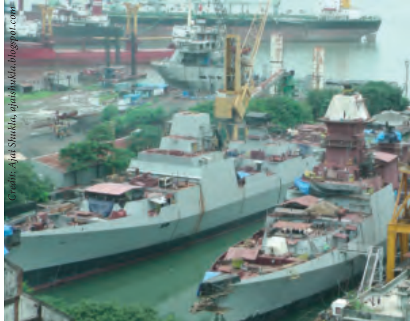
The 2 nd (background) and 3 rd (foreground) Project 15A Kolkata-class destroyers being built at Mazagon Docks, Mumbai, 24 April 2008. The destroyers are being indigenously designed, developed and built for the Indian Navy, and are the first using modular construction techniques.
