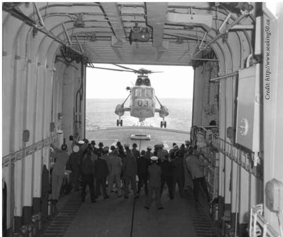
This photo illustrates early tests of the Helicopter Hauldown and Rapid Securing Device – the innovative Beartrap system.
