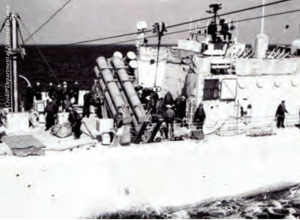
HMCS Terra Nova's Harpoon missile launchers were installed hastily before deployment to the Persian Gulf.
