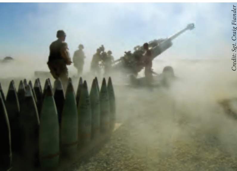
Gunners from X Battery, 5 e Régiment d'artillerie légère du Canada, conduct a fire mission against a Taliban position with an M777 155mm Howitzer.
