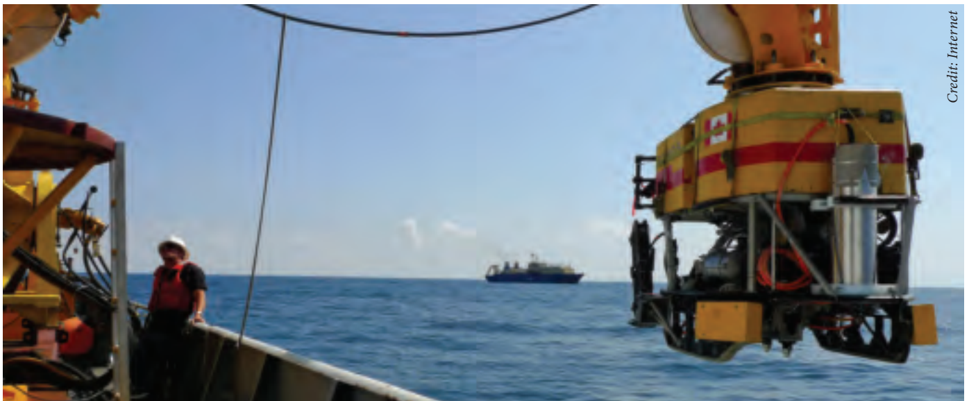
Crews lower the undersea robot ROPOS to assist in the installation of Neptune Canada's Endeavour node.
