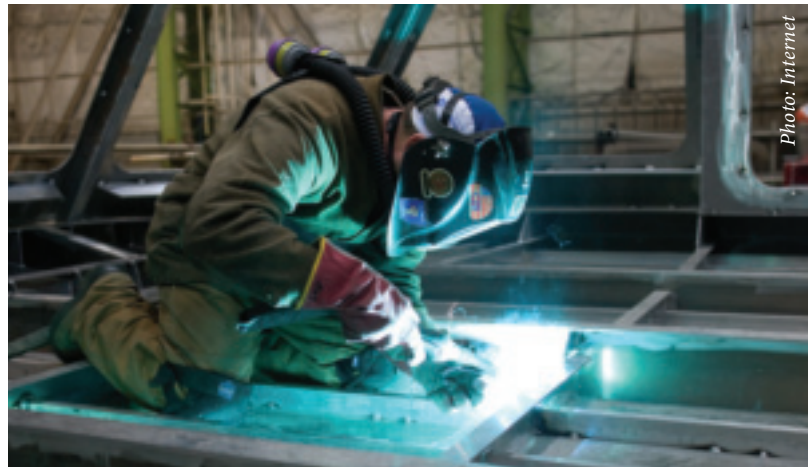
A welder works in the wheelhouse of one of the Mid-Shore Patrol Vessels under construction for the Canadian Coast Guard.
