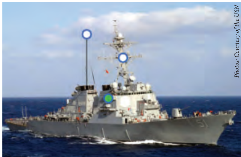
Possible deceptive lighting configuration shown on Arleigh Burke -class destroyer. The ways in which a warship can be deceptively lit are limited only by the crew's imagination, and the resourcefulness of the shipwrights and riggers who implement the deceptive lighting plan.
