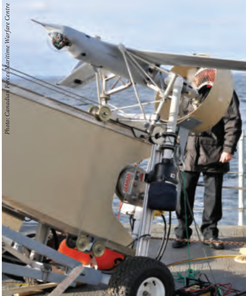
ScanEagle UAV in launch position onboard HMCS Glace Bay prior to sea trials and evaluation by Canadian Forces Maritime Warfare Centre personnel, 28 October 2009.
