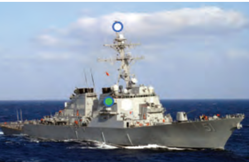
American Arleigh Burke -class destroyer, starboard aspect, with masthead light and starboard running light locations emphasized.
