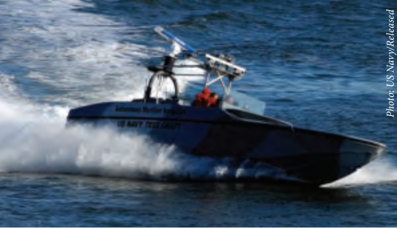
US Navy demonstration of a fully autonomous USV depicting the use of navigation systems to patrol and scan designated areas for intruders using onboard sensors and obstacle avoidance software, 14 January 2009.
