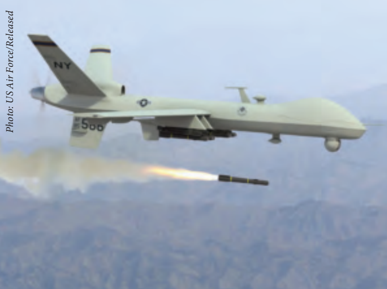
US Air Force MQ-9 (Reaper) unmanned aerial vehicle carries up to 3,750 pounds of laser-guided munitions, giving ground commanders both excellent situational awareness and choice about the amount of force to use.
