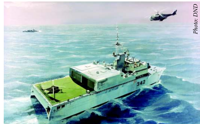
The need for new ships creates new intellectual challenges as innovative hull forms and propulsion systems are proposed in vessels such as the small waterplane area twin hull – the 'SWATH' – ship.
