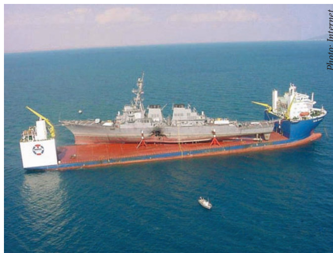
MV Blue Marlin carrying USS Cole back to the United States after a devastating water-borne suicide attack on the ship killed 17 sailors and tore a 40 by 40 foot hole in its side.
