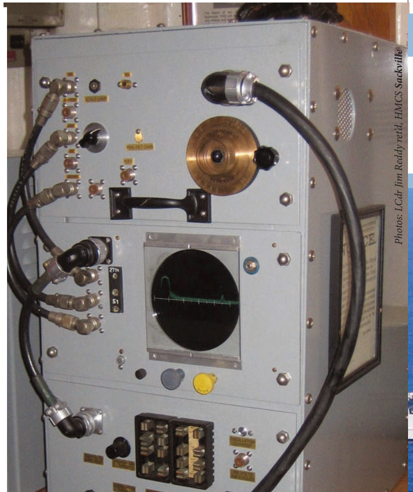
Newly restored Type 271 radar onboard HMCS Sackville.
