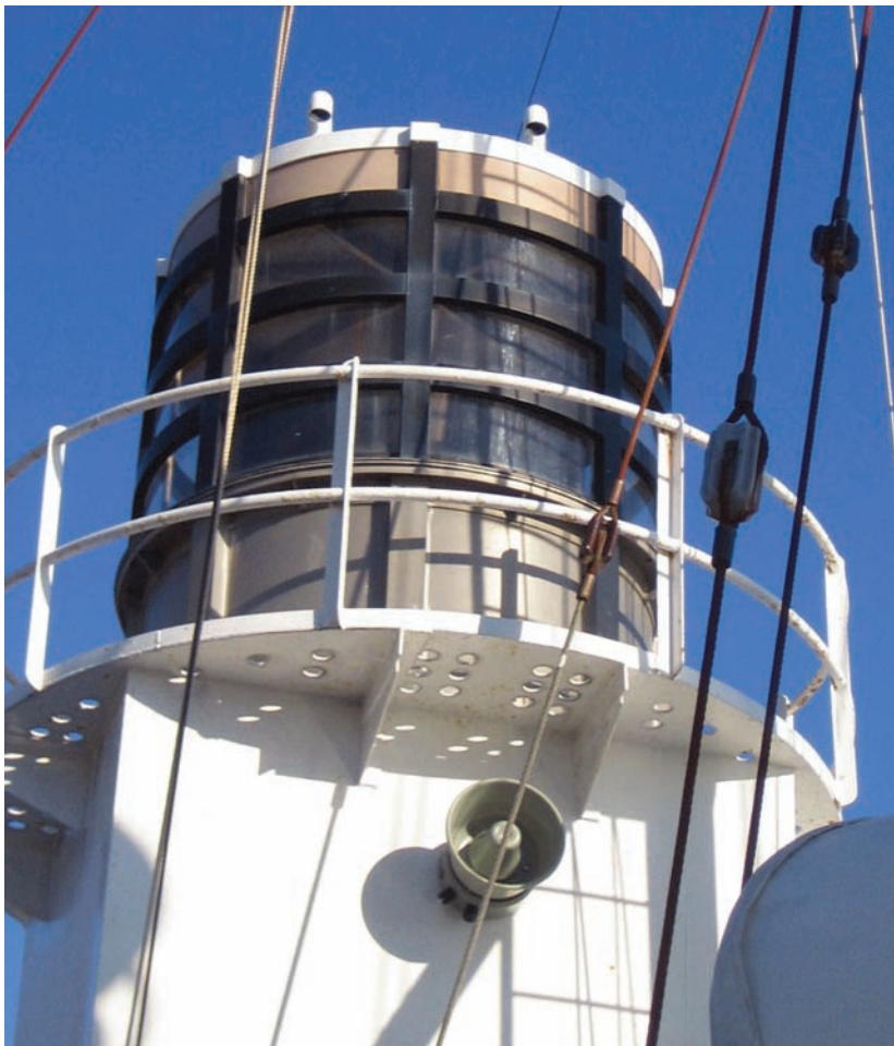
Sackville's Type 271 radar lantern was usually covered while the ship was alongside as a security measure to prevent enemy agents from obtaining its dimensions to determine its operating frequency.
