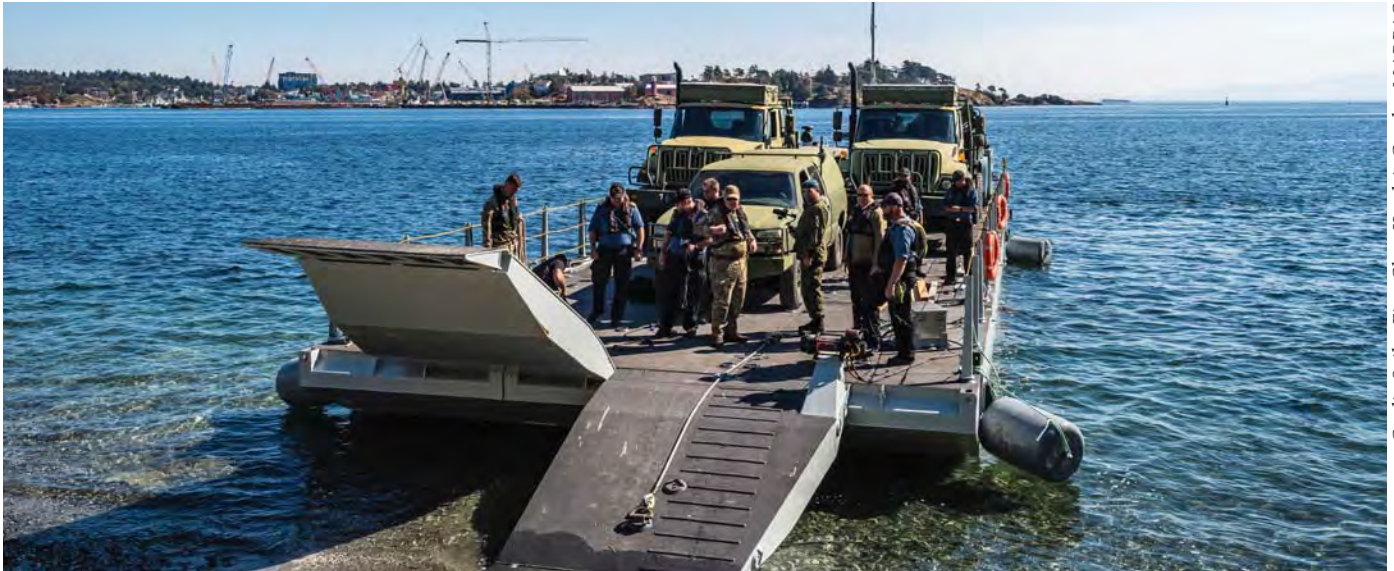
In Esquimalt, BC, Canadian sailors train in 2022 using the RCN's new sea-to-shore connector, a modular, self-propelled barge designed to support the future Joint Support Ships.
