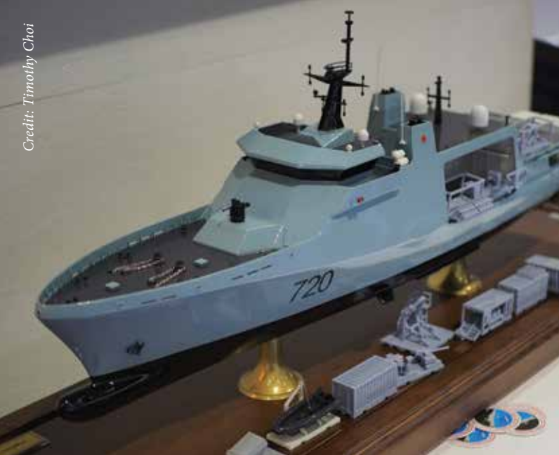
A model of the 'Vigilance' offshore patrol vessel proposed by Vard and SH Defence to replace the Kingston -class. It incorporates a larger hull and modular equipment spaces to reflect expanded mission sets and operating areas.
