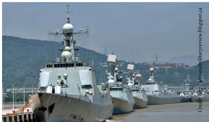
Chinese Type 052C air defence guided-missile destroyers can carry 48 HHQ-9 long-range surface-to-air missiles to provide area defence to the Chinese carrier fleet.
