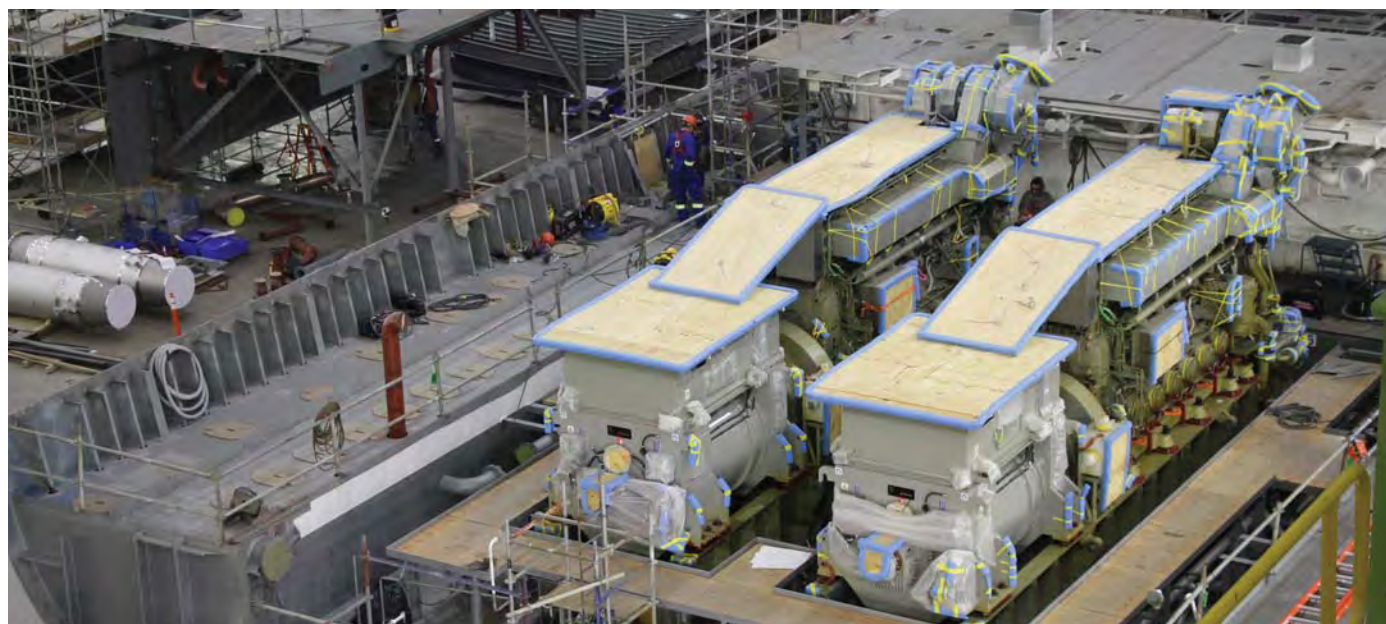
The first two of four main propulsion diesel engines and generators are installed on HMCS Harry DeWolf at Halifax Shipyard, 10 June 2016.
