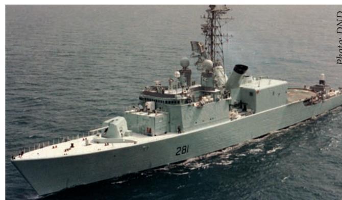
HMCS *Huron* in the Persian Gulf in 1991 in pre-TRUMP configuration with additional self-protection systems needed for Operation Friction.
