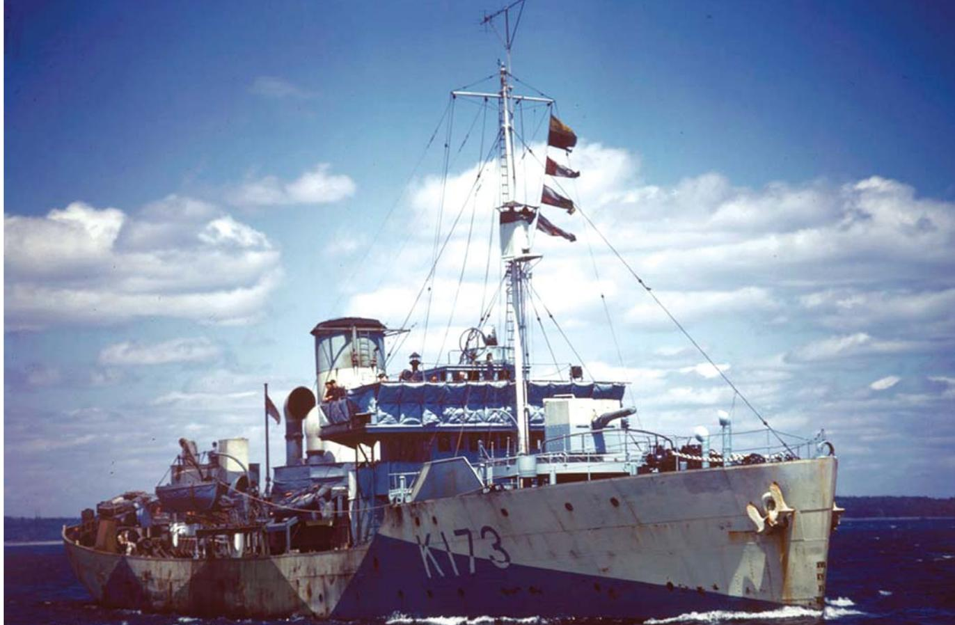
*Flower-class corvette HMCS Weyburn, circa 1942. Illustrating the somewhat ad hoc approach to corvette modernization, Weyburn is shown here with the triangular Canadian-developed SW1C radar at the top of the mast and wider bridge wings, yet lacking some of the newer modifications such as an extended forecastle.*
