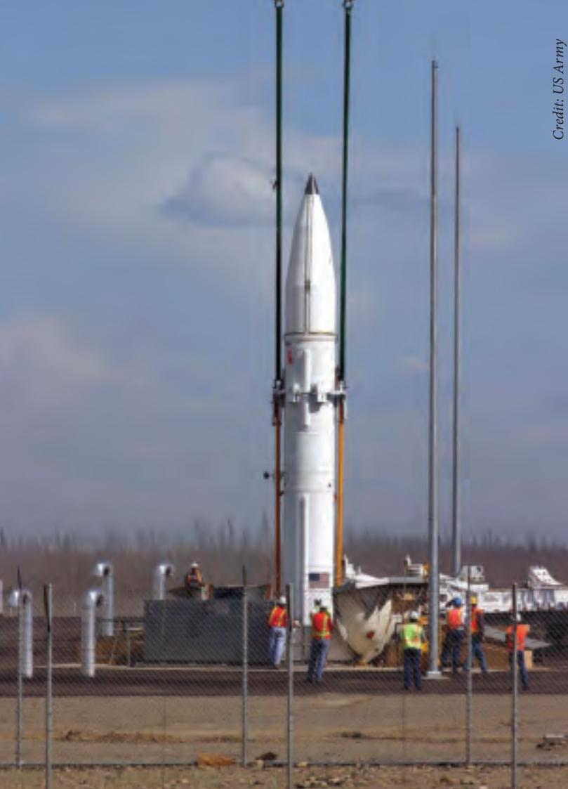
*The first ground-based interceptor is lowered into its silo at the missile defence complex at Fort Greely, Alaska, 22 July 2004. The interceptor is designed to destroy incoming intercontinental ballistic missiles before they reach US airspace.*
