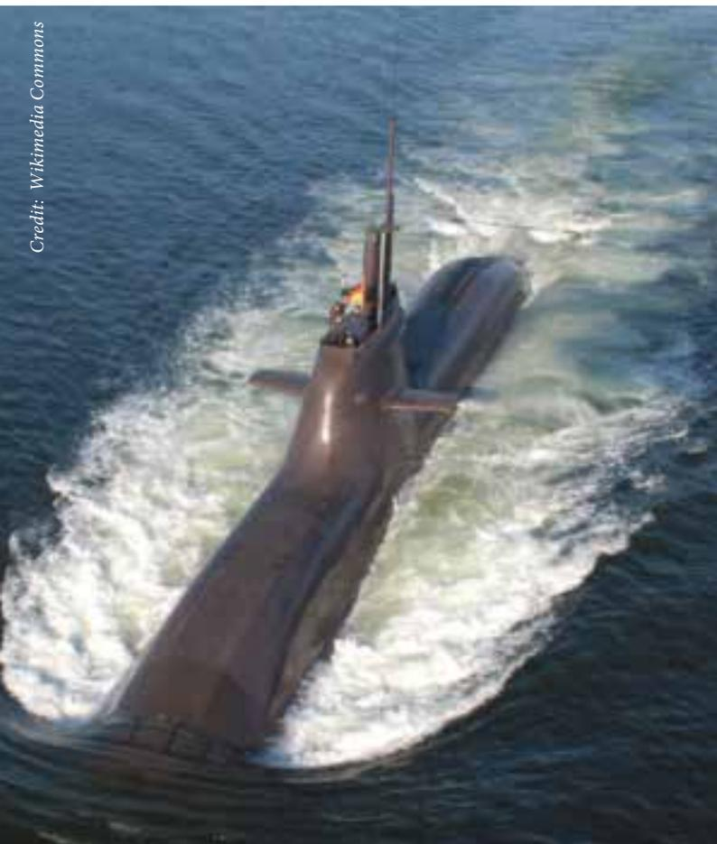
*U-32 (S182), the second Type 212A submarine of the German Navy, is powered by one diesel engine and an electric motor driven by two fuel cells. Photo 8 March 2010.*
